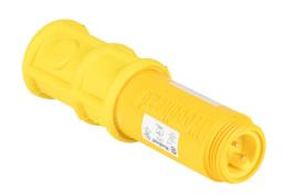
Molex pendant switch, nitrile rubber/PVC, single pushbutton, flush, yellow, snap action, (1) N.C. contact(s), 7/8in - 16 UN2 2-pin male. Requires 7/8in - 16 UN2 2-pin connection cable.
