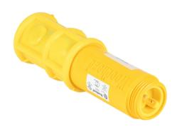
Molex pendant switch, silicone rubber/PVC, single pushbutton, flush, yellow, snap action, (1) N.O. contact(s), 7/8in - 16 UN2 2-pin male. Requires 7/8in - 16 UN2 2-pin connection cable.
