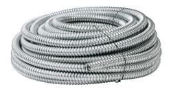
Southwire Gaflex flexible metallic conduit, reduced wall steel, 3/4in trade size, UL-1 Listed, 100ft/30.4m coil length.
