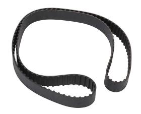
SureMotion timing belt, 3/8in L pitch, 1in wide, 144 tooth, 54in pitch length (circumference), neoprene, fiberglass reinforced.
