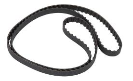
SureMotion timing belt, 3/8in L pitch, 1/2in wide, 144 tooth, 54in pitch length (circumference), neoprene, fiberglass reinforced.
