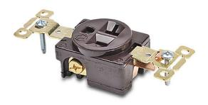
Bryant industrial heavy duty single straight blade receptacle, 20A, 125 VAC, 1-phase, 2-pole, 3-wire, NEMA 5-20, nylon housing, brown.
