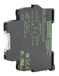
Murrelektronik optocoupler relay, 35mm DIN rail mount, fingersafe, 10-53 VDC input voltage, SPST, (1) N.O. MOSFET, 10A contact rating, 5-48 VDC load voltage, screw terminal(s), LED indicator(s).
