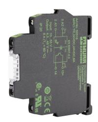
Murrelektronik optocoupler relay, 35mm DIN rail mount, fingersafe, 10-53 VDC input voltage, SPST, (1) N.O. MOSFET, 6A contact rating, 5-48 VDC load voltage, screw terminal(s), LED indicator(s).
