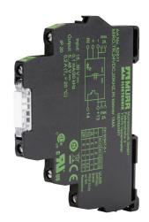
Murrelektronik optocoupler relay, 35mm DIN rail mount, fingersafe, 15-30 VDC input voltage, SPST, (1) N.O. transistor, 0.2A contact rating, 5-48 VDC load voltage, screw terminal(s), LED indicator(s).
