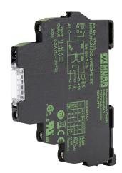
Murrelektronik optocoupler relay, 35mm DIN rail mount, fingersafe, 10-53 VDC input voltage, SPDT, (1) N.O., (1) N.C. transistor, 0.5A contact rating, 5-48 VDC load voltage, screw terminal(s), LED indicator(s).
