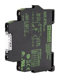
Murrelektronik optocoupler relay, 35mm DIN rail mount, fingersafe, 4-5.5 VDC input voltage, SPST, (1) N.O. MOSFET, 2A contact rating, 5-48 VDC load voltage, screw terminal(s), LED indicator(s).
