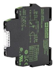
Murrelektronik optocoupler relay, 35mm DIN rail mount, fingersafe, 10-48 VDC input voltage, SPST, (1) N.O. MOSFET, 2A contact rating, 5-48 VDC load voltage, screw terminal(s), LED indicator(s).
