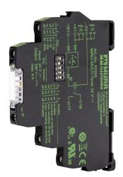
Murrelektronik multi-mode relay timer, 0.1 to 300 seconds selectable timing range, 24 VDC operating voltage, 6A contact rating, (1) SPST timed relay output(s), 35mm DIN rail mount, screw terminal(s).
