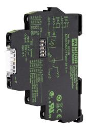
Murrelektronik multi-mode relay timer, 0.1 to 300 seconds selectable timing range, 24 VDC operating voltage, 6A contact rating, (1) SPST timed relay output(s), 35mm DIN rail mount, screw terminal(s).
