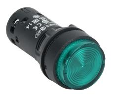
IDEM compact pushbutton, IP65, 22mm, momentary, LED, (1) N.C. contact(s), plastic base, plastic bezel, Operator: green, extended, 29mm, round, plastic, 24 VAC/VDC, full voltage. For use with UGB series universal gate boxes.
