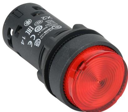
IDEM compact pushbutton, IP65, 22mm, momentary, LED, (1) N.C. contact(s), plastic base, plastic bezel, Operator: red, extended, 29mm, round, plastic, 24 VAC/VDC, full voltage. For use with UGB series universal gate boxes.
