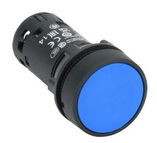
IDEM compact pushbutton, IP65, 22mm, momentary, (1) N.O./(1) N.C. contact(s), plastic base, plastic bezel, Operator: blue, flush, 29mm, round, plastic. For use with UGB series universal gate boxes.
