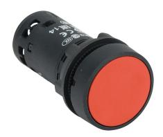
IDEM compact pushbutton, IP65, 22mm, momentary, (1) N.O./(1) N.C. contact(s), plastic base, plastic bezel, Operator: red, flush, 29mm, round, plastic. For use with UGB series universal gate boxes.
