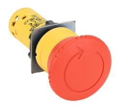
IDEM compact emergency stop pushbutton, IP54, 22mm, twist-to-release, (2) N.C. contact(s), plastic base, plastic bezel, Operator: red, mushroom, 40mm, round, plastic. For use with UGB series universal gate boxes.
