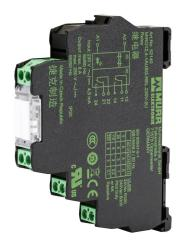
Murrelektronik interface relay, 35mm DIN rail mount, finger-safe, 230 VAC/VDC coil voltage, DPDT, (2) N.O., (2) N.C., 6A contact rating, 250 VAC/VDC load voltage, screw terminal(s), LED indicator(s).
