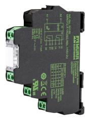
Murrelektronik interface relay, 35mm DIN rail mount, finger-safe, 110 VAC/VDC coil voltage, DPDT, (2) N.O., (2) N.C., 6A contact rating, 250 VAC/VDC load voltage, screw terminal(s), LED indicator(s).
