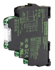
Murrelektronik interface relay, 35mm DIN rail mount, finger-safe, 24 VAC/VDC coil voltage, DPDT, (2) N.O., (2) N.C., 6A contact rating, 250 VAC/VDC load voltage, screw terminal(s), LED indicator(s).
