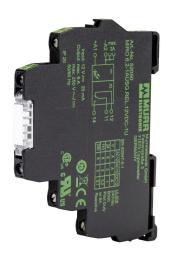
Murrelektronik interface relay, 35mm DIN rail mount, finger-safe, 12 VDC coil voltage, SPDT, (1) N.O., (1) N.C., 6A contact rating, 250 VAC/VDC load voltage, screw terminal(s), LED indicator(s).
