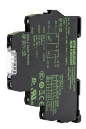
Murrelektronik interface relay, 35mm DIN rail mount, finger-safe, 230 VAC/VDC coil voltage, SPDT, (1) N.O., (1) N.C., 6A contact rating, 250 VAC/VDC load voltage, screw terminal(s), LED indicator(s).
