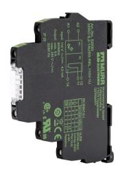
Murrelektronik interface relay, 35mm DIN rail mount, finger-safe, 110 VAC/VDC coil voltage, SPDT, (1) N.O., (1) N.C., 6A contact rating, 250 VAC/VDC load voltage, screw terminal(s), LED indicator(s).
