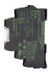
Murrelektronik interface relay, 35mm DIN rail mount, finger-safe, 24 VAC/VDC coil voltage, SPDT, (1) N.O., (1) N.C., 6A contact rating, 250 VAC/VDC load voltage, isolation disconnect, screw terminal(s), LED indicator(s).
