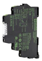
Murrelektronik interface relay, 35mm DIN rail mount, finger-safe, 24 VAC/VDC coil voltage, SPST, (1) N.O., 6A contact rating, 250 VAC/VDC load voltage, H-O-A toggle switch, screw terminal(s), LED indicator(s).
