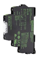
Murrelektronik interface relay, 35mm DIN rail mount, finger-safe, 24 VAC/VDC coil voltage, SPDT, (1) N.O., (1) N.C., 6A contact rating, 250 VAC/VDC load voltage, screw terminal(s), LED indicator(s).
