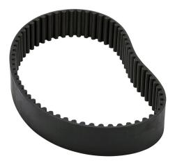
SureMotion timing belt, 8mm 8M pitch, 30mm wide, 65 tooth, 520mm pitch length (circumference), neoprene, fiberglass reinforced.
