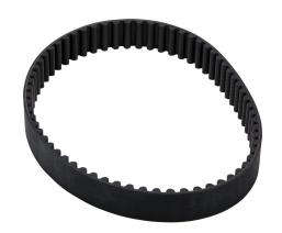
SureMotion timing belt, 8mm 8M pitch, 20mm wide, 65 tooth, 520mm pitch length (circumference), neoprene, fiberglass reinforced.
