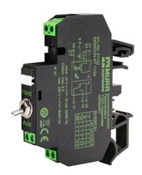
Murrelektronik interface relay, 35mm DIN rail mount, finger-safe, 24 VAC/VDC coil voltage, SPDT, (1) N.O., (1) N.C., 8A contact rating, 250 VAC/VDC load voltage, H-O-A toggle switch, screw terminal(s), LED indicator(s).
