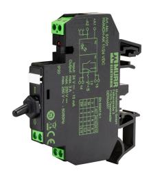
Murrelektronik interface relay, 35mm DIN rail mount, finger-safe, 24 VDC coil voltage, SPST, (1) N.O., 3A contact rating, 250 VAC/ VDC load voltage, manual-auto toggle switch, screw terminal(s), LED indicator(s).
