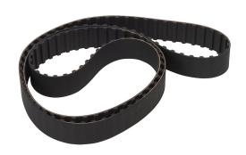
SureMotion timing belt, 3/8in L pitch, 1in wide, 136 tooth, 51in pitch length (circumference), neoprene, fiberglass reinforced.
