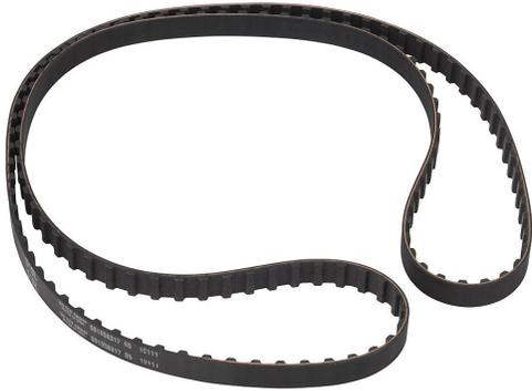
SureMotion timing belt, 3/8in L pitch, 1/2in wide, 136 tooth, 51in pitch length (circumference), neoprene, fiberglass reinforced.
