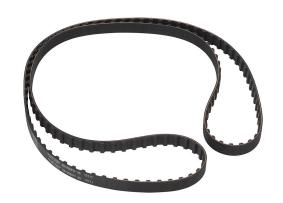
SureMotion timing belt, 3/8in L pitch, 1/2in wide, 136 tooth, 51in pitch length (circumference), neoprene, fiberglass reinforced.
