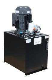
Bucher T-Series hydraulic power unit, 6.8 GPM, 2800 psi, 30 gal reservoir, 10hp, 230/460 VAC operating voltage.
