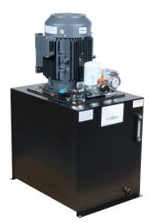
Bucher T-Series hydraulic power unit, 6.8 GPM, 1600 psi, 30 gal reservoir, 7-1/2hp, 230/460 VAC operating voltage.
