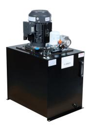
Bucher T-Series hydraulic power unit, 5 GPM, 1500 psi, 30 gal reservoir, 5hp, 230/460 VAC operating voltage.
