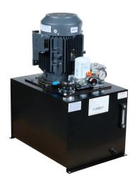
Bucher T-Series hydraulic power unit, 3.8 GPM, 3000 psi, 20 gal reservoir, 7-1/2hp, 230/460 VAC operating voltage.
