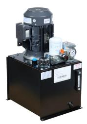
Bucher T-Series hydraulic power unit, 2 GPM, 2200 psi, 10 gal reservoir, 3hp, 230/460 VAC operating voltage.
