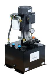
Bucher M-Series hydraulic power unit, 2 GPM, 1500 psi, 8 gal reservoir, 2hp, 115/208-230 VAC operating voltage.
