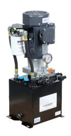
Bucher M-Series hydraulic power unit, 1 GPM, 3000 psi, 4 gal reservoir, 2hp, 115/208-230 VAC operating voltage.
