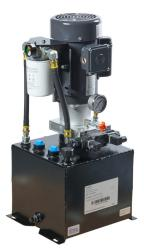
Bucher M-Series hydraulic power unit, 1.5 GPM, 1500 psi, 6 gal reservoir, 1-1/2hp, 115/208-230 VAC operating voltage.
