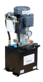
Bucher M-Series hydraulic power unit, 1 GPM, 1500 psi, 4 gal reservoir, 1hp, 115/208-230 VAC operating voltage.
