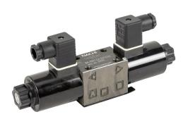
Bucher solenoid valve, D03, 4-port (4-way), 3-position, center open, double solenoid, cast iron body, momentary manual override, Cv=13.2, 24 VDC.
