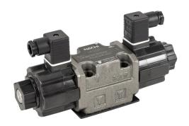
Bucher solenoid valve, D05, 4-port (4-way), 3-position, center tandem, double solenoid, cast iron body, momentary manual override, Cv=26.4, 120 VAC.
