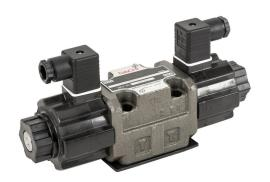
Bucher solenoid valve, D05, 4-port (4-way), 3-position, center open, double solenoid, cast iron body, momentary manual override, Cv=42.2, 120 VAC.
