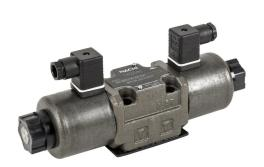
Bucher solenoid valve, D05, 4-port (4-way), 3-position, center tandem, double solenoid, cast iron body, momentary manual override, Cv=26.4, 24 VDC.
