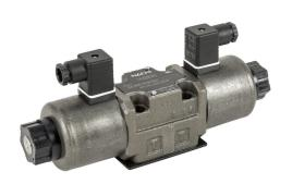
Bucher solenoid valve, D05, 4-port (4-way), 3-position, center open, double solenoid, cast iron body, momentary manual override, Cv=42.2, 24 VDC.
