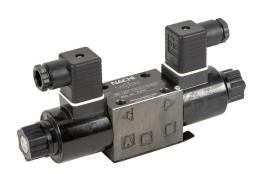
Bucher solenoid valve, D03, 4-port (4-way), 3-position, center float, double solenoid, cast iron body, momentary manual override, Cv=21.1, 120 VAC.
