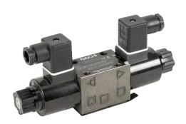
Bucher solenoid valve, D03, 4-port (4-way), 3-position, center closed, double solenoid, cast iron body, momentary manual override, Cv=26.4, 120 VAC.
