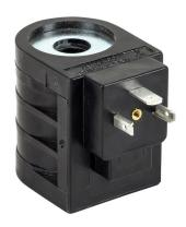
Bucher solenoid coil, replacement, 24 VDC, 22W, DIN 43650 connector. For use with Bucher solenoid valve 51020850999.
